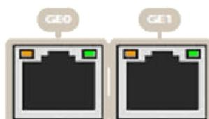
Fig. 3: Gigabit Ethernet interface LEDs
